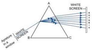
19. Fig. shows a thin beam of white light from a source S striking on one face of a prism.
