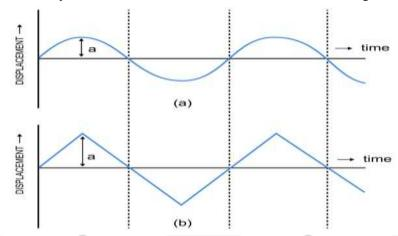
The figure above shows the wave forms of two sounds of same loudness (i.e., same amplitude) and same pitch (i.e., same frequency), but emitted by two different sources.
